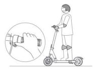
5.3 When the scooter starts to coasting, put both feet on the deck, and press the thumb shift accelerator when you can keep balance (the accelerator start to work once the coasting speed exceeds 3km/h).
