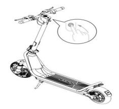
3.4 After the assembly, turn on the power button to test whether the electric scooter works properly.
