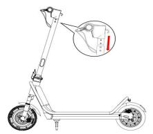
3.2 Firmly connect the wires inside the handle and the stem. Be aware of the correct orientation. Attach the handlebar to the handlebar stem.
