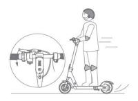
5.4 Release the thumb shift accelerator to slow down.
