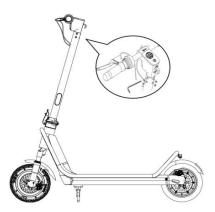
3.3 Take the hexagon wrench and M5 screws(6 pcs) out from The Accessories package, tighten two screws onto each of the Three sides of the Handlebar stem with the hexagon wrench.
